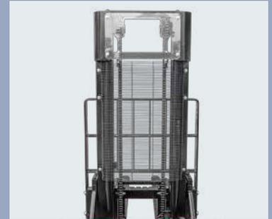
Mast can offer better rigidity and stability in comparison with C-shaped steel channels
