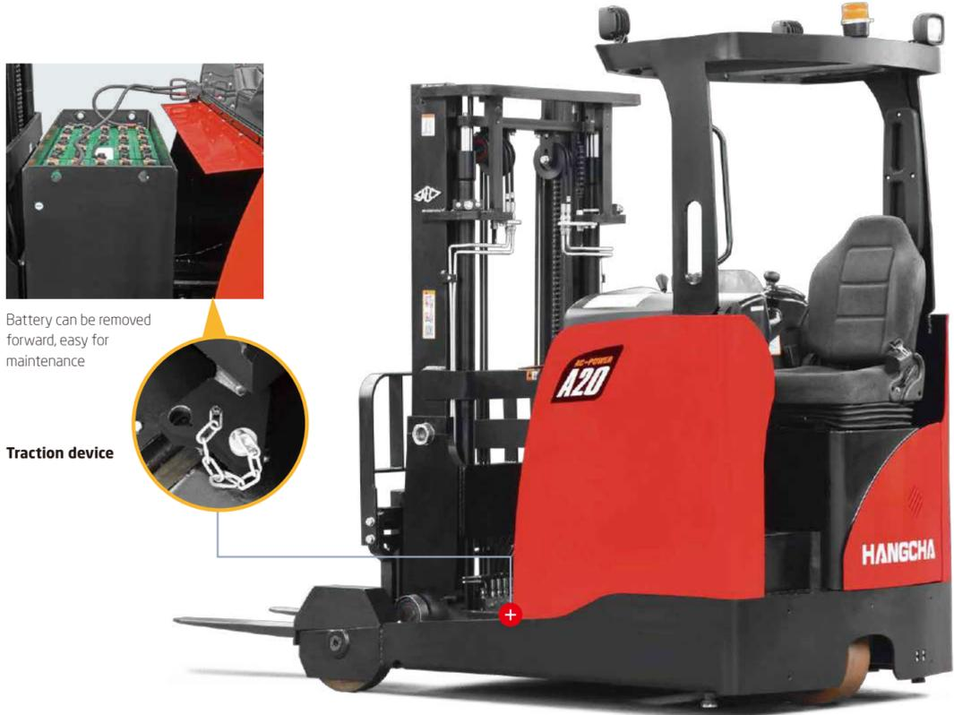
Battery can be removed forward, easy for maintenance
