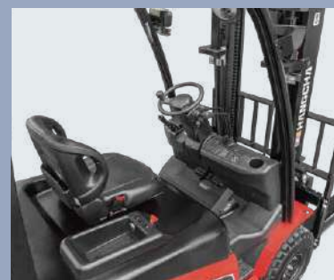
Fully closed operation plate space, tilting cylinder and flat bottom plate, providing more comfortable and safe operation
