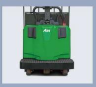
The roomy, low step height, platform is designed to reduce operator fatigue. The optional cushioned knee pads allow the operator to adjust there stance throughout the shift. This creates a more comfortable operating experience.
