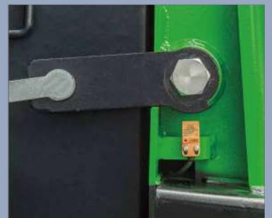
The tow tractor has a safety feature where it can only travel if the battery locking pin is correctly rotated.
