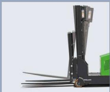
The mast tilting function makes loading and unloading pallets easy.
