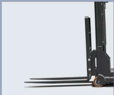
Mast speed will automatically reduce when the fork is lowered to a height less than 3.9" from ground.
