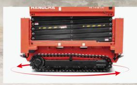
The steering proportional deceleration and electronic differential function can make the machine pivot steering.
