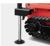
Equipped with one key outrigger leveling function, automatically adjust the frame to the level state, hydraulic outrigger to enhance the stability of the equipment. At the same time, it can also operate a single outrigger to meet the operation requirements under special working conditions.
