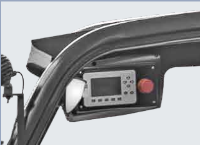
The dashboard in the driver's cab is placed overhead and can be seen when the driver lift her/his head, and the function buttons can be pressed easily
