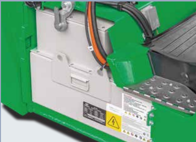
The packs can be easily removed by a manual or electric cart, and can be repaired and maintained conveniently
