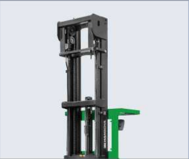
With a safety factor of 10, the mast chain is equipped with a chain safety switch.
