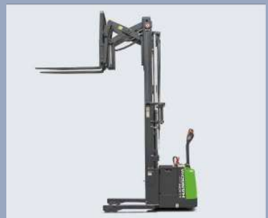
Travel speed is reduced automatically when the forks are lifted past a specified height.
