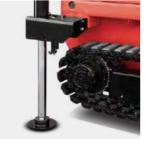
Equipped with one key outrigger leveling function, automatically adjust the frame to the level state, hydraulic outrigger to enhance the stability of the equipment. At the same time, it can also operate a single outrigger to meet the operation requirements under special working conditions.
