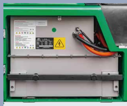
A laterally-removed roller-equipped battery compartment
