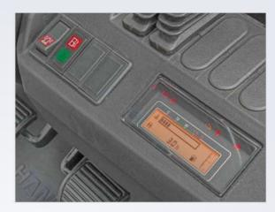
The newly developed LCD instrument display has additional functions and offers more stable performance. Important information including the running status of the entire truck and a check engine light can be displayed. This allows the operator to easily understand the status of the truck for easy maintenance.
