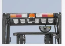
LED lights are used throughout the entire truck. The lights are energy-efficient, have a longer service life, and offer a significant increase in performance.
